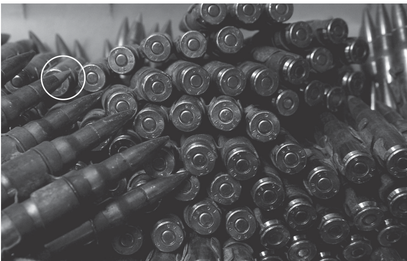
Figure 2.26 Belted 7.62×51mm cartridges. Note the orange-painted tip, circled, indicating that the cartridge is a tracer. (U.S. Air Force image; photographer Technical Sgt. Jeremy Lock, USAF.)
